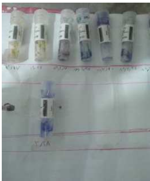
Figure 1. TST test of pilot autoclave of Amin Hospital
